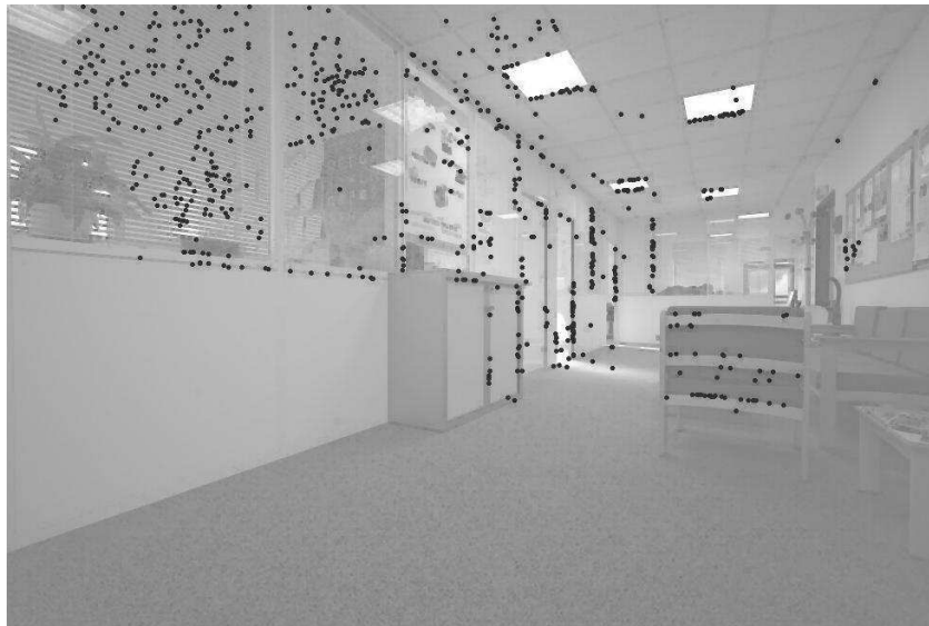
Fig. 4. Flies resulting of one particular run of the Fly algorithm, here projected on the left image (printout contrast has been reduced in order to enhance the visibility of flies).
